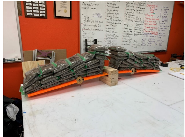
Figure 36: Wing Loaded to n = 5 g.
