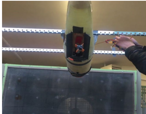
Figure 34: Deployment and Retraction Testing at Wind Tunnel.
