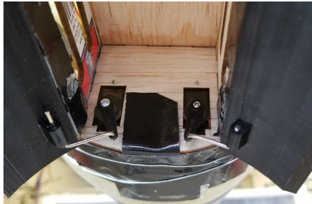
Figure 18: Bomb Bay Door Servo Configuration.
