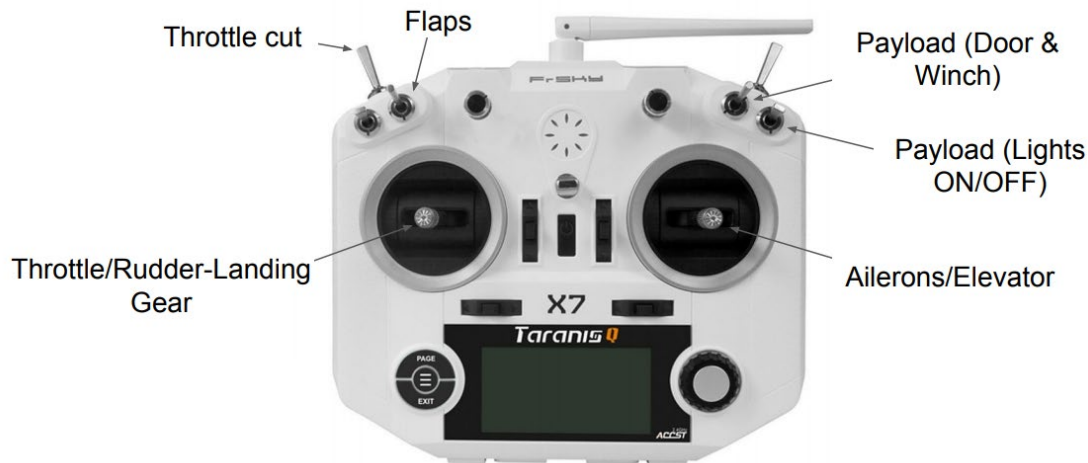
Figure 30: Transmitter Switch and Control Layout.
