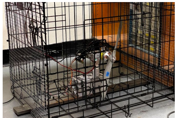
Figure 35: Competition Motor on Thrust Stand.
