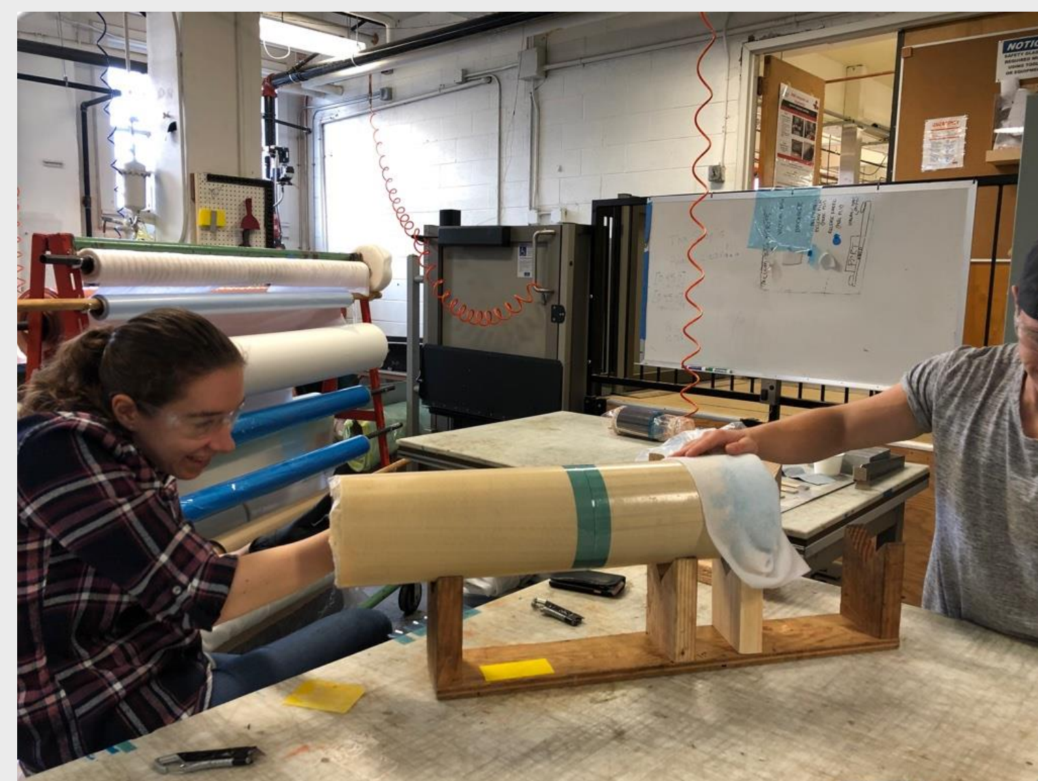
Figures 2: Manufacturing the nose cone joint tube
