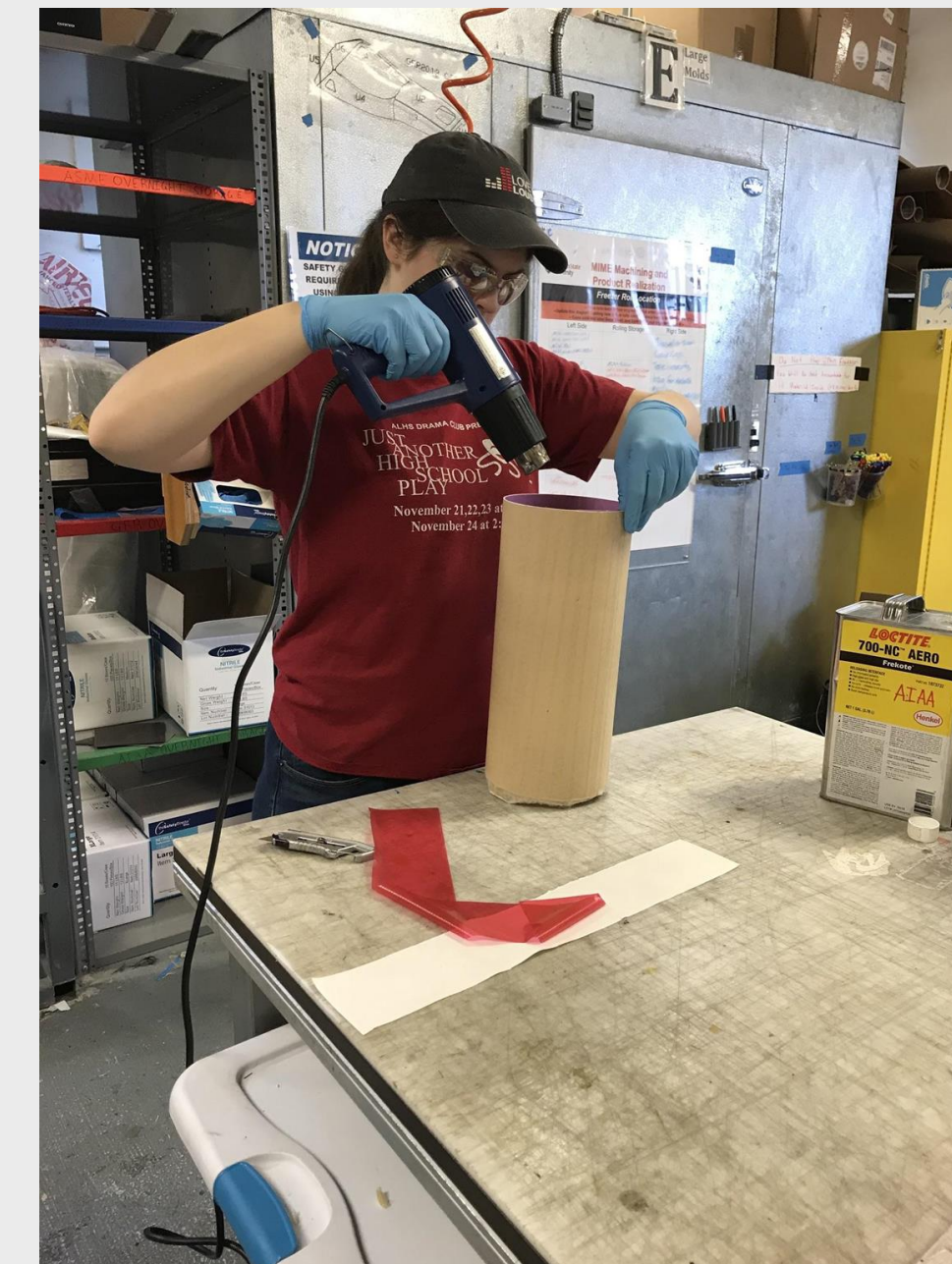
Figure 3: Heating up film adhesive for the joint tube
