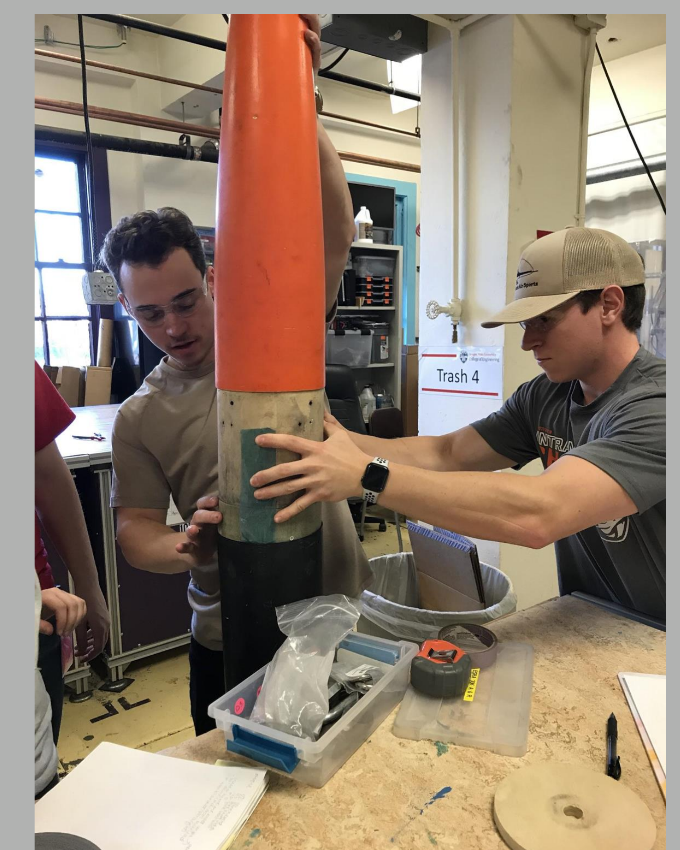
Figure 6: Attaching the nosecone during integration tests
